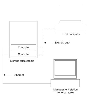
Figure 25. Direct (out-of-band) managed storage subsystems
